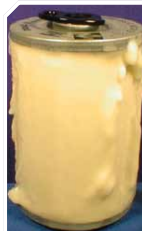
Crystal growth / Filter blocking
