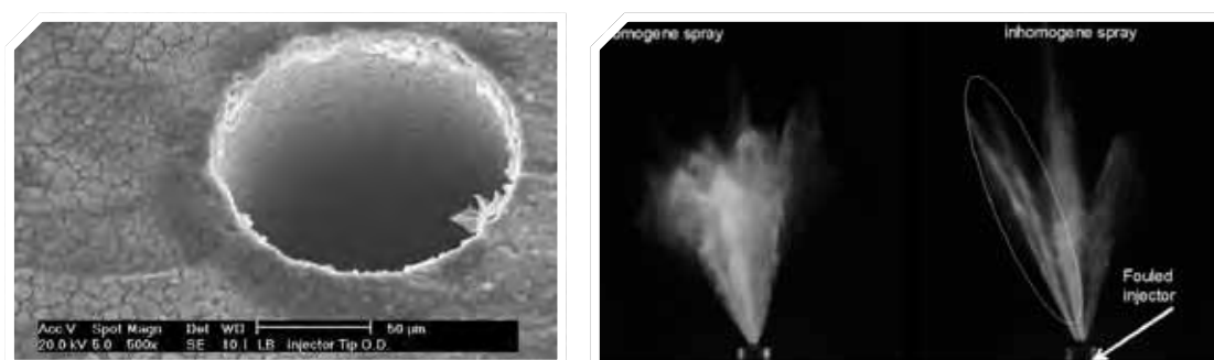
Injector deposit images / Fuel spray
